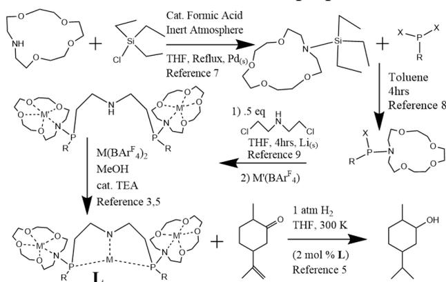
**Scheme 1:** Synthetic route for **L**. X= Halide; M= Co (II), Ir (II), Re (II), Rh (II); M'=Na<sup>+</sup>, Li<sup>+</sup>, Ca<sup>2+</sup>; R=Ph, Me, Cy.
